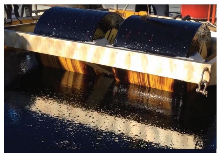
Alaska North Slope crude oil/i-Petrogel solution is recovered by an Elastec TDS 118 oleophilic drum skimmer. The recovered oil/i-Petrogel solution contains almost no water and can be refined using regular refining processes. Overall, i-Petrogel technology potentially provides a comprehensive solution for combating crude oil spills in open waters, with dramatic reduction in environmental impacts. Photo: Courtesy Mike Chung
