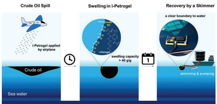
The *i*-Petrogel technology potentially provides a comprehensive solution for combating crude oil spills in open waters, with dramatic reduction of environmental impact. Illustration: Courtesy Mike Chung
