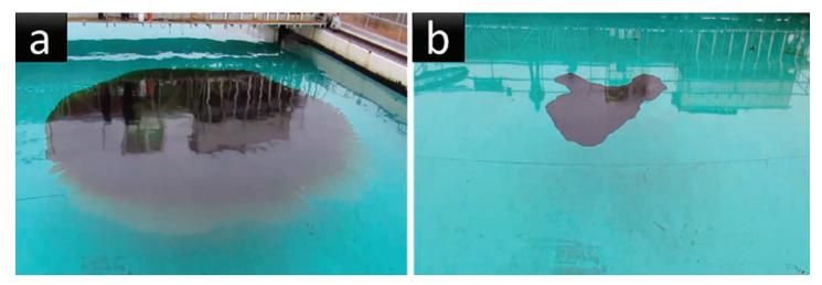
Two gallons of fresh Alaska North Slope oil released into tank (a) diffused quickly from the spill site. The same Alaska North Slope oil, treated with i-Petrogel before releasing (b), showed no significant spreading, The oil/i-Petrogel solution formed a clear boundary to water, indicating no free oil. Photos: Mike Chung
